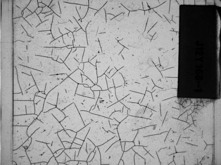
**Figure 2.** *Example image showing loss of adhesion at multiple interfaces on a steam clean test panel*
